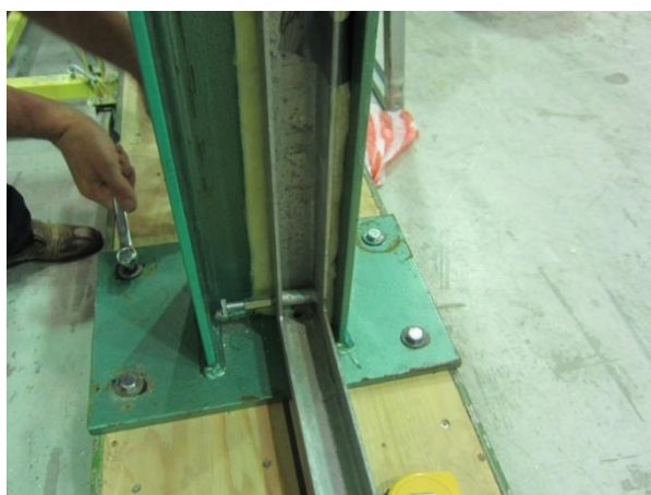
Photo 1. Steel frame for installation of planks to test opening
